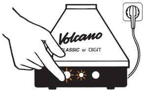
1. Switch heat on (takes 3-5 min.)
